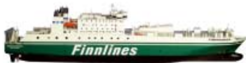
MS Finnhansa (II) , (1994–) Combi ro-ro 3,200 lane metres, 114 passenger berths, speed 20 knots. Built in Poland.
